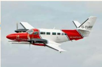
Wing span and fuselage dimensions are strikingly close, the main design difference is with the Pilatus incorporating a single engine whereas the Cessna goes with the more conventional approach of using twin power plants.
